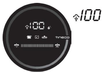
After switching to the Steaming mode, the number starts to read. After reaching 100, the nozzle starts to spray steam.
